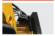
The RT726H model uses a hydraulic motor and can be ordered for either standard or high flow skid loaders.
