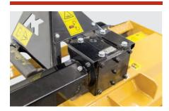
A powerful gear box transfers power from the tractors 540RPM PTO to the chain drive delivering a tine speed 211RPM.
