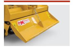
An adjustable floating deflector helps to control displaced soil as it is processed by the tines. Raise or lower it to get the desired amount of surface compaction for your application.
