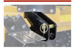
Standard on the MK Rotary Tiller is the adjustable 3PH mount. This allows you to offset the tiller while hooked up to your 3PH, giving you even more control over the placement of your tiller for those hard to reach to places.
