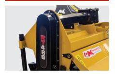
The chain drive equipped on the Rotary Tiller is self lubricated, removing the need for lubricating the chain drive before every use. The base of the casing is filled with oil that lubricates the chain as it passes through the bottom of the chain drive.
