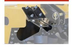
Each side of the Rotary Tiller comes equipped with safety guards to help prevent limbs from entering into the rotor and tines during operation.
